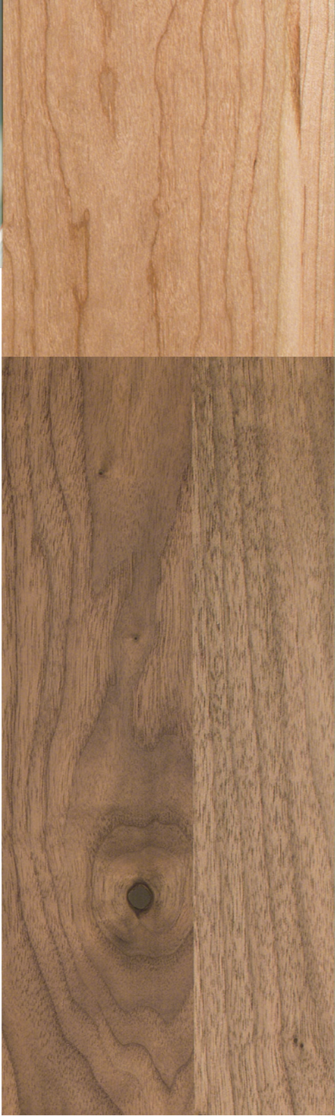
To prevent scrap wood from going to waste, the Steelcase operations team saw an opportunity for a new material offering: planked veneer. Production of this new offering—that celebrates the uniqueness of wood through seaming together different scrap veneers side by side—has saved $1 million and over 400 trees.
